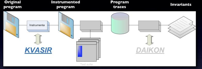
The program is instrumented to trace the content of each variable during its execution
